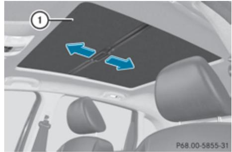
Roller sunblind ① for the panorama louvred sliding sunroof or the fixed panorama roof shields the vehicle interior from sunlight.
