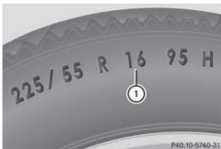
Rim diameter ① is part of the tyre size and can be found on the tyre sidewall.
