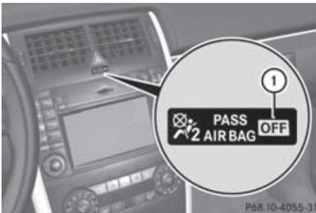
The automatic child seat recognition sensor system on the front-passenger seat detects whether a special Mercedes-Benz child seat with automatic child seat recognition has been fitted there. In this case,
