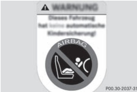
If your vehicle does not have automatic child seat recognition<sup>7</sup> on the front-passenger seat, this is indicated by a special sticker. The sticker is affixed to the side of the dashboard on the front-passenger side. The sticker is visible when you open the front-passenger door.
