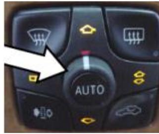
**Figure 14 Left AUTO Air Delivery Button Extended In Manual Mode**
