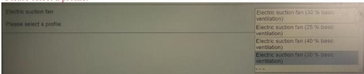
Coding options are: ‘Electric suction fan (25% basic ventilation)’, ‘Electric suction fan (40% basic ventilation)’, ‘Electric suction fan (30% basic ventilation)’ or ‘---’.
