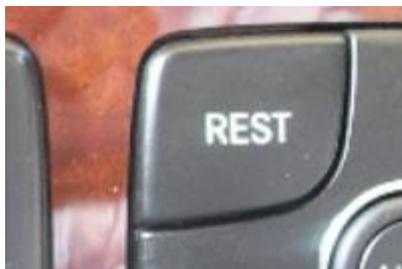
Figure 3 Residual Heat and Ventilation (REST) Button
