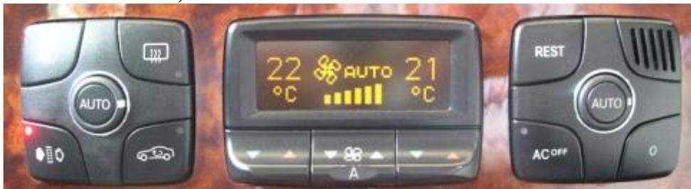
**Figure 13 Both ACC AUTO Air Delivery Knobs Pressed In**
