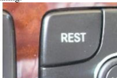
**Figure 5 Recirculate and Residual Heat and Ventilation (REST) Buttons**
