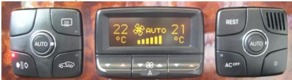
Figure 9 Both ACC AUTO Knobs Pressed In
