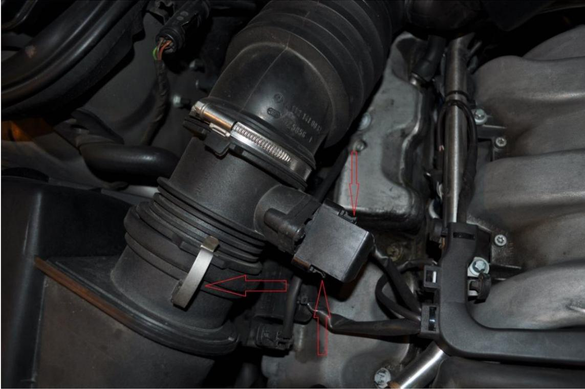
Release the 6 clips on the air cleaner cover and remove the cover.
