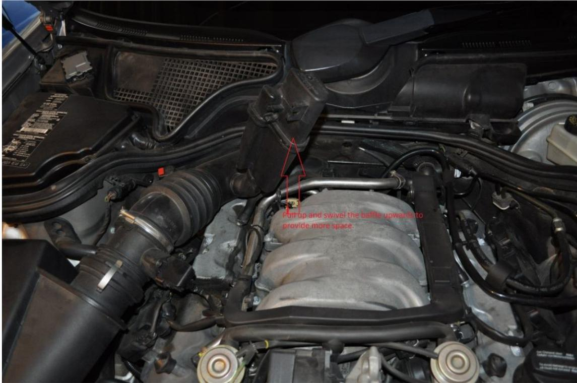
Release the silver clip marked with arrow, as well as the one on the opposite side of the intake pipe. Remove the plug from the MAF by pressing down where the arrows indicate and pulling back on the plug.
