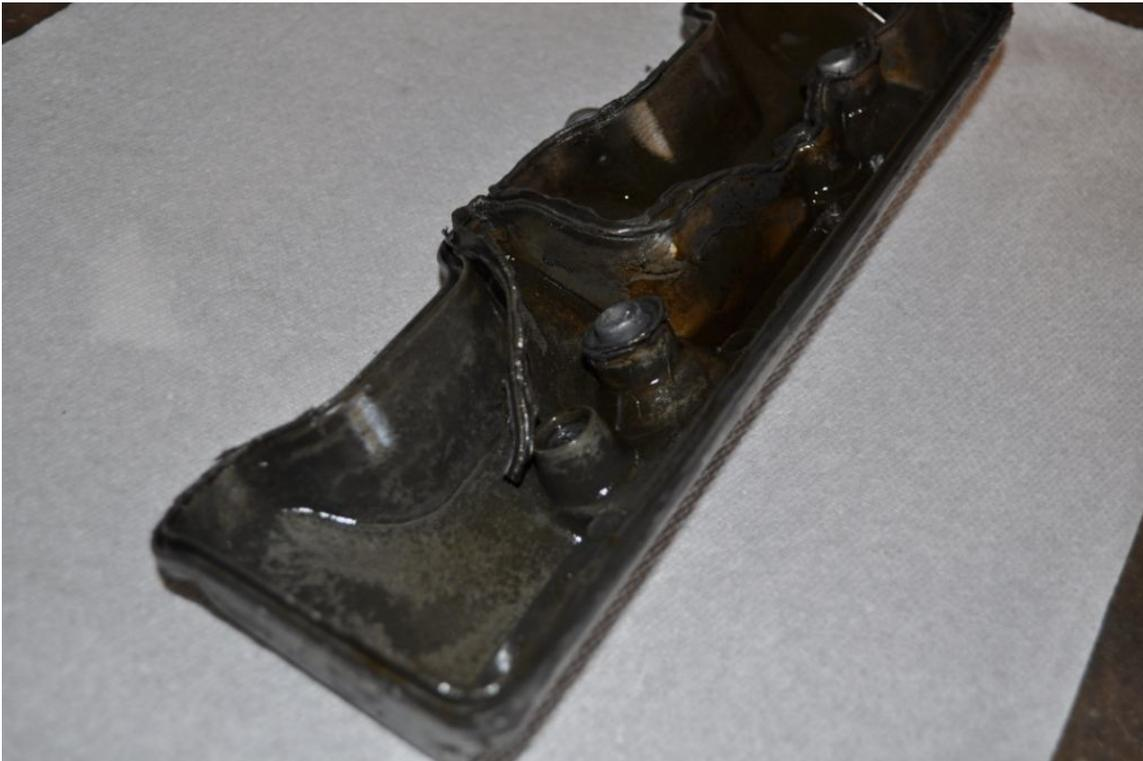
And the top of the cam cover, where the breather cover has been removed. Also still nice and clean and no gunk. Notice the stud in the lower left corner that can be used for leverage to remove the breather cover.
