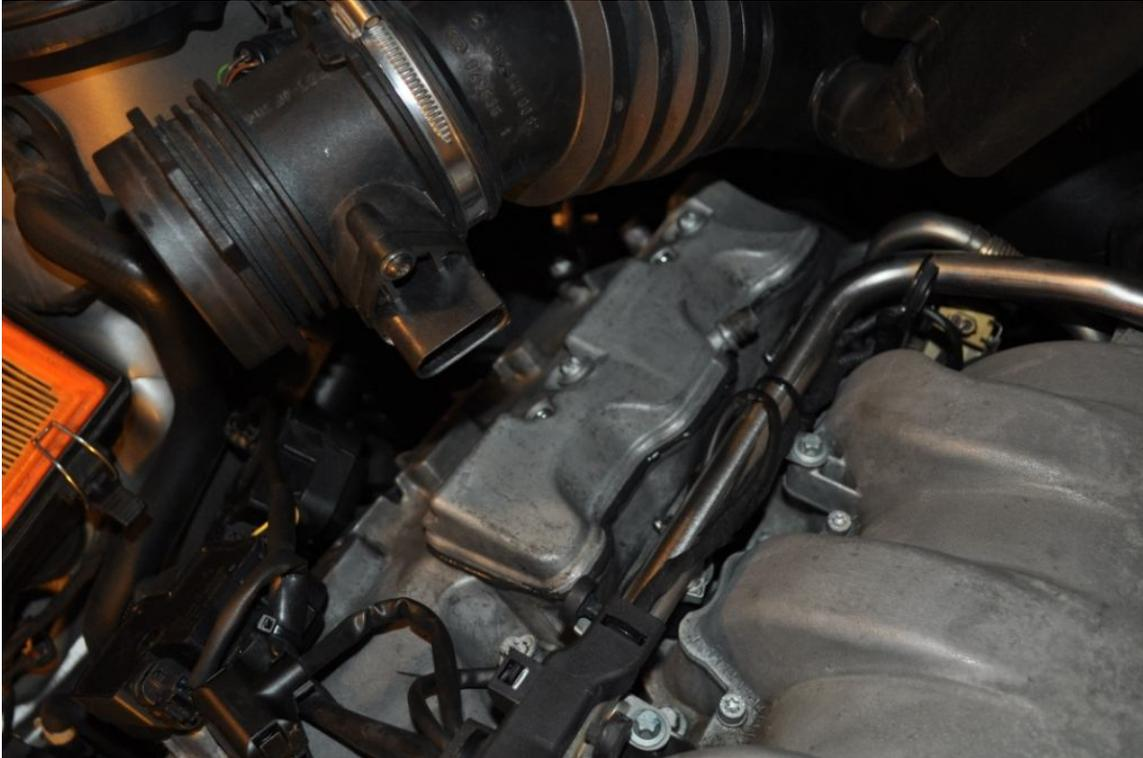
Replacing the rest of the pieces removed is just the reverse of the removal process. One tip I would like to share: When replacing the bolt next to the transmission tube that is holding the air pipe, first swivel down the baffle and push it down over the connector. You have to work on feeling and in a limited space to replace the bolt and the baffle helps to position the intake pipe so that the bolt can take.
