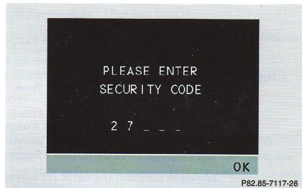
If the power supply to the MCS has been interrupted, "PLEASE ENTER SECURITY CODE" will appear on the display when it is next switched on. The MCS will only work after the five digit code has been entered using the number keypad.
