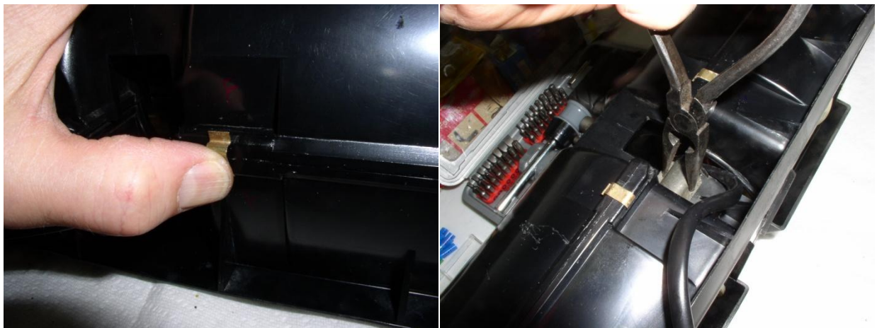
Figure 17. Install eight small and two large housing clips. The large clips should be spread by a pair of snap ring pliers to make installing them easier and avoid stressing the plastic housing.
