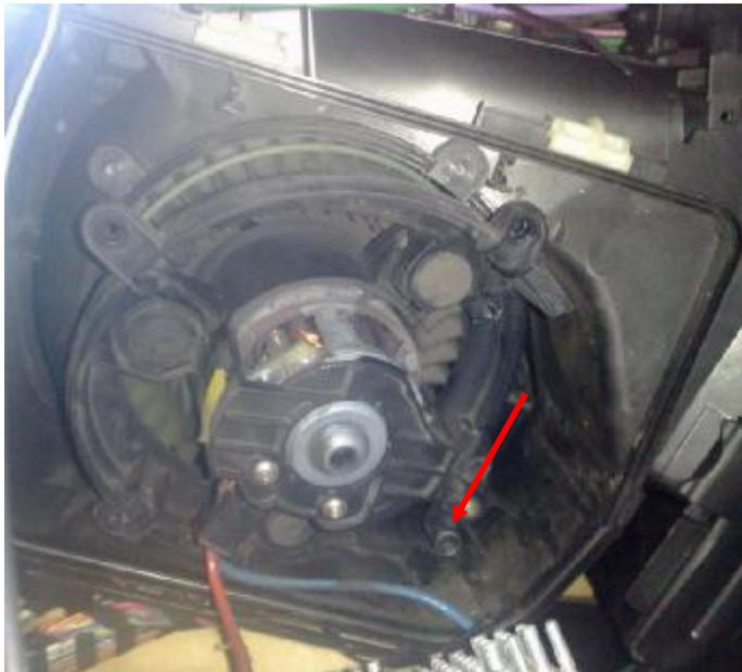
Remove the power cable and gently remove the motor from the car and bring it inside to work on it. Remove the 2 screws retaining the plastic cover in place and remove it.
