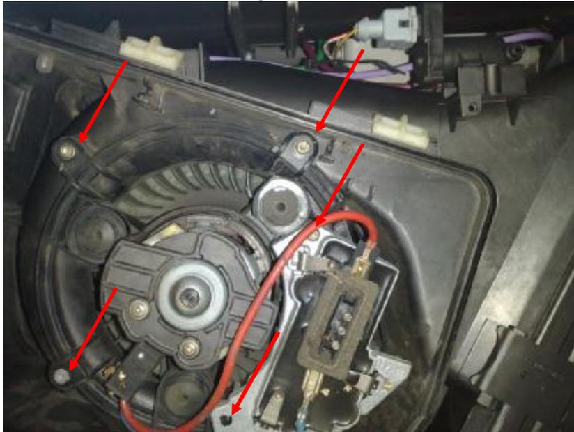
Once the regulator is removed the fourth torx screw beneath it holding the motor in place can be removed.
