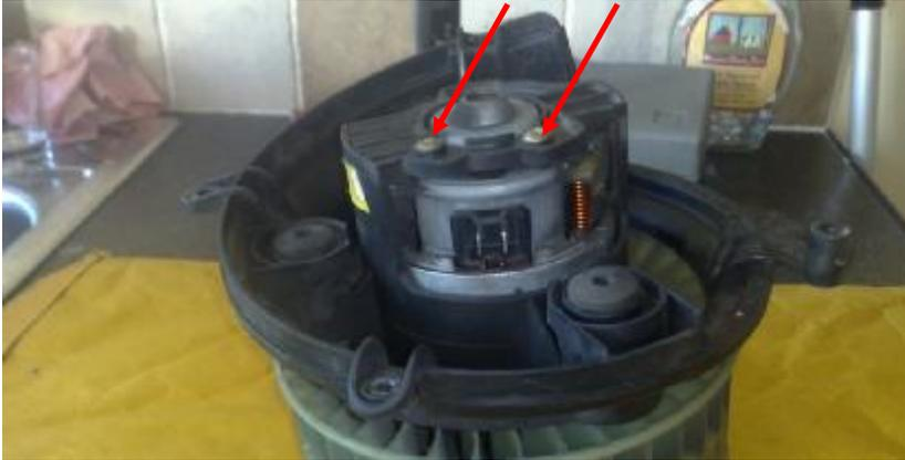
Remove the clips holding the springs and brushes in place with a screwdriver.
