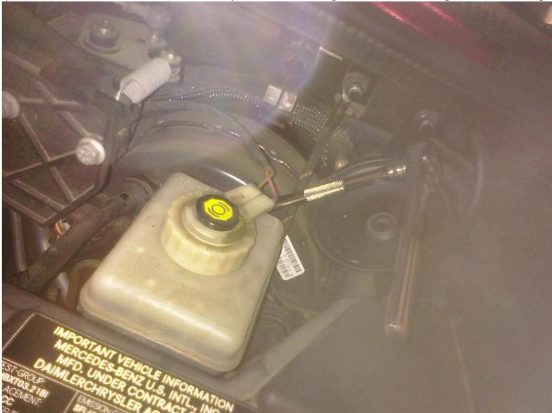
Get on top of the engine and put a flashlight right there behind this brake fluid reservoir. It will look like on the other picture I have of the CPS without the plug on it. It will help if you have the new plug in your hand. See the pic of the old and new CPS's.
