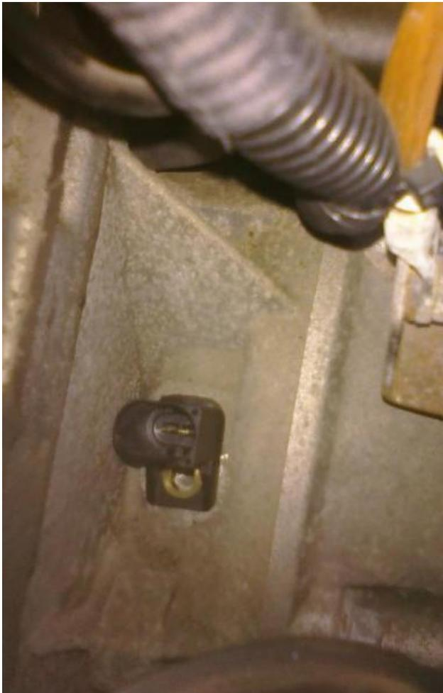
8. Place the CPS plug back on the sensor.
