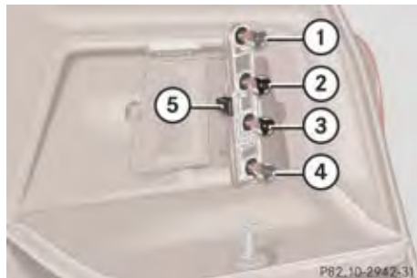
Right-hand lamp cluster (left-hand lamp cluster mirror image)
