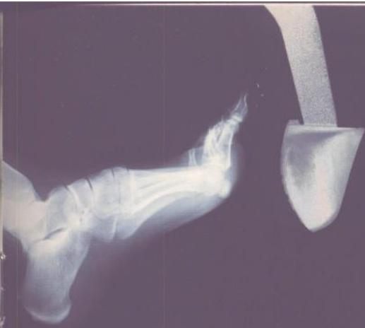
To reduce the risk of injury to the driver's lower legs and feet, the Mercedes-Benz brake pedal assembly tends to **pivot forward** in a severe offset frontal impact, away from the driver's feet. Underhood components are **staggered** to help prevent intrusion into the cabin.
