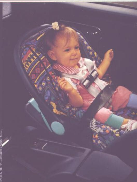
The SLK is the first production car to feature **Mercedes-Benz BabySmart™** technology, a system that helps protect your child from the forces of a deploying front air bag. Whenever a Mercedes-Benz accessory child seat is properly installed in the SLK, the BabySmart system automatically turns off the passenger's front air bag.<sup>1</sup>
