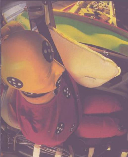
Full frontal impacts have received much attention lately. But offset frontal collisions, in which impact forces are neither perpendicular to nor uniformly spread across the width of the car, continue to be frequent and injurious. Years ago, Mercedes-Benz instituted **offset collision tests** for all of its cars, resulting in safety systems which are better prepared for the real world.
