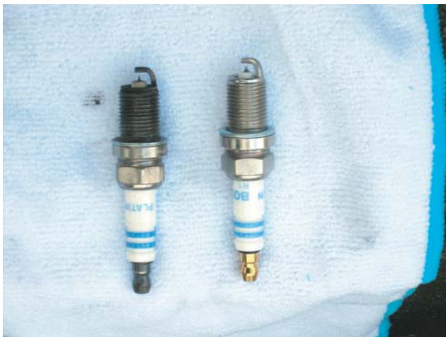
Fig. 6. Old and new spark plugs. I used OEM spark plugs, as seen in Fig. 7.
