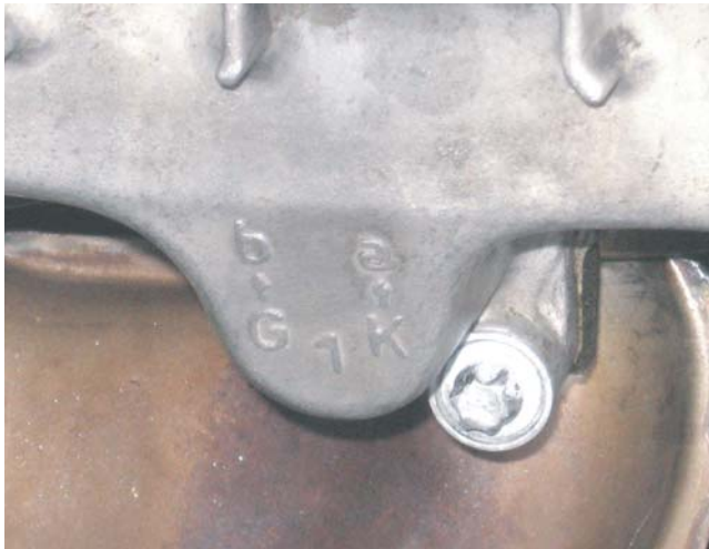
Fig. 5. The engine has embossed lettering to show which boot goes where.
