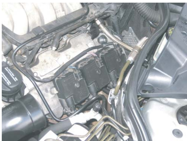
Fig. 3. Spark plugs on driver's side with wires and harnesses intact.
