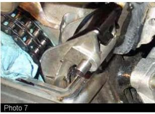
This pin is often difficult and must be removed to get the head off. We use a small slide hammer of our own manufacture. The center of the pin is threaded, and it can be pulled with a bolt and various cylindrical spacers such as the socket in Photo 8.
