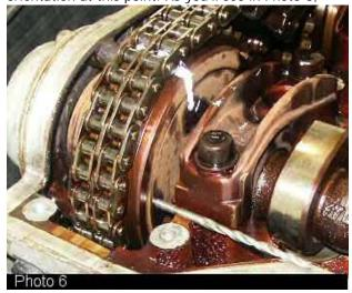
we've made a mark across the chain and gear. This is a cross-check for use in final assembly of the intake cam timing adjuster. The proper location of the cam is indicated by a 4mm drift ({any 4mm rod can be used} see the drill in photo 6). In the proper position, the drift fits into the hole in the flange and sits on the parting surface of the head. The same arrangement exists on the exhaust side.
