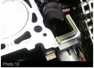
a dab of M-B p/n 001 989 61 20 10 should be placed before assembly. There are other similar sealants that make a sticky flexible seal, but the M-B variety works well. No sealant should be used on the "U" seal (except where the dab sits at the ends of the "U").
