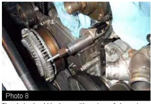
The chain should be hung with a piece of shop wire, and the tensioner should be removed.
