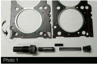
It's my diagnosis that part of the long-range problem is that the head gasket recedes under the head after a period of time. Over time, the resilience of that spongy gasket can't keep up with the receding gasket and a leak is formed.
