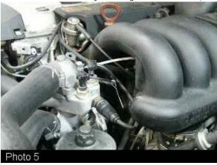
We remove the head with the top/plastic manifold, separating it at those two large hoses.
