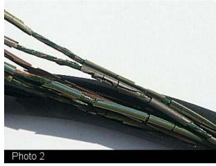
The act of doing this work will ruin a harness that is falling apart. It's very expensive, and something you won't need at the end of the job. The harness problems occur on the engine harness on the engine, the engine harness on the body and the harness from the throttle actuator. Be sure to check the state of these harnesses before selling this job on 1993-'95 models.
